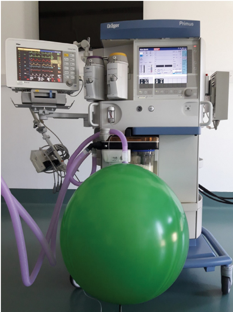
Figure 4: Reservoir bag's safety function – the maintenance of a constant pressure in the respiratory system (example in the figure: pressure inside the reservoir bag: 34 cm H 2 O, diameter: 66 cm, volume: 150 litres).
