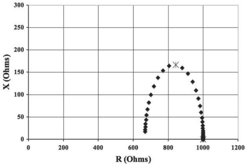
**Figure 3:** Idealized “Cole-Cole plot” for the circuit shown in Figure 1 with generic values:  $R_e = 1000$  Ohms,  $R_i = 2000$  Ohms and  $C = 1$  nanoFarad.
