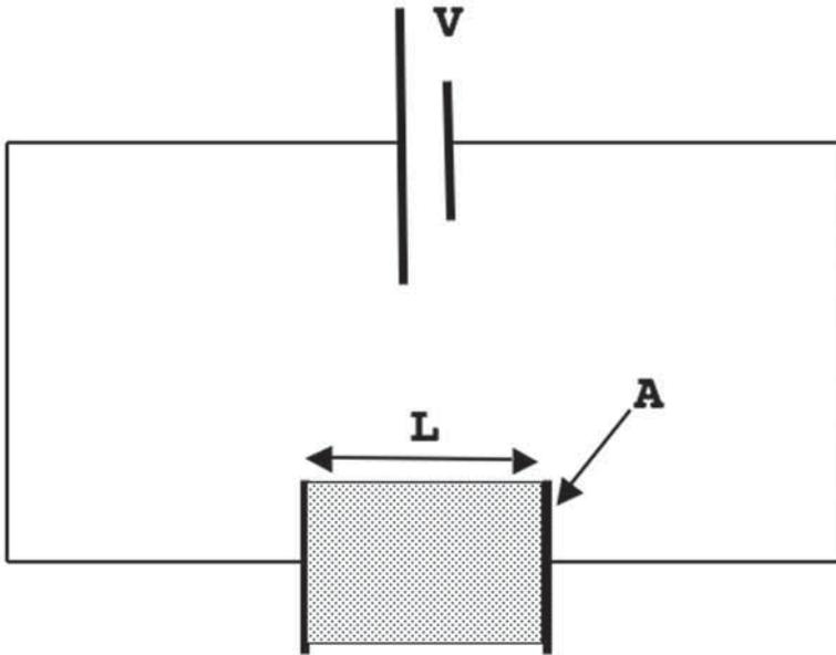
**Figure 1:** A sample of material with length  $L$  connected to a battery of voltage  $V$ . The sample has an area  $A$ , perpendicular to the plane of the page.
