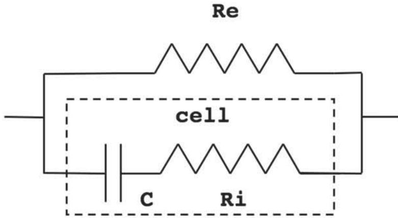
**Figure 2:** Circuit diagram for the Fricke model. The dashed line encloses the body of the cell. C represents the transmembrane capacitance and Ri is the resistance of the intracellular medium. Re is the resistance of the extracellular medium.
